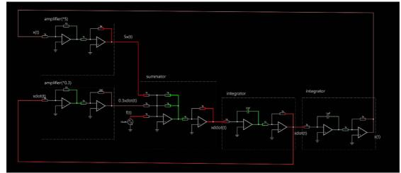
Solving second-order differential equations with different coefficients can be achieved by changing the resistance value of the resistors and bypassing some inverters. computers are still in charge of simulations and controls in aircrafts and industrial processes where reliability and reaction speed are the first concerns.
