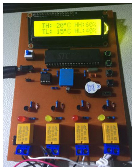
Figure 15 setting the temperature exceeds the upper limit
