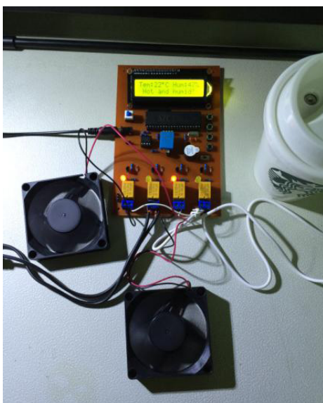
Figure 21 Results diagram when temperature exceeds the upper limit and humidity exceeds the upper limit
