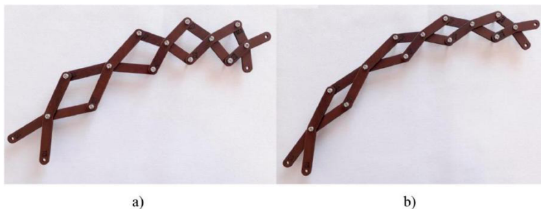
Fig. 7 The unfolding process of angulated scissor structure: a) deployed state; b) fully deployed state [9].
