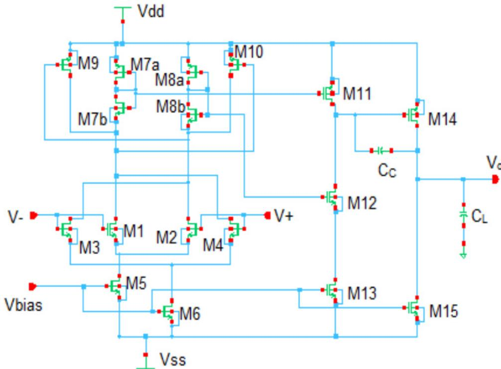
Fig. 2 A highly linear and high gain operational amplifier [6].
