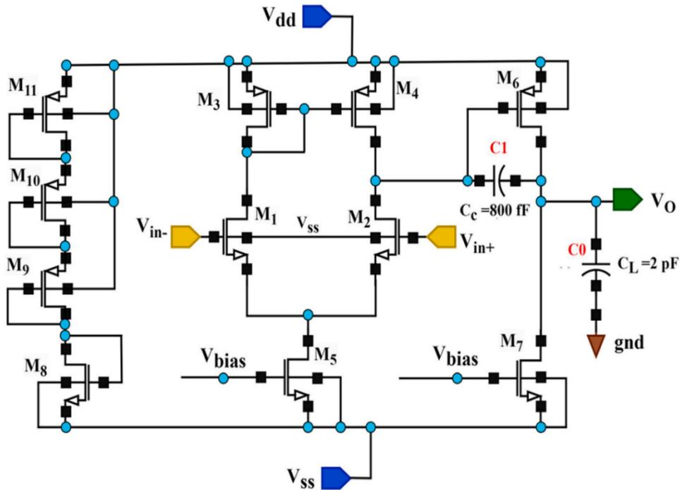
**Fig. 1 A CMOS operational amplifier design [4].**
