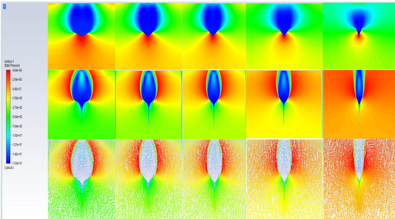
**Fig. 5 From left to right, the pressure field, velocity field and velocity vector field for elevation angles of 30, 45, 50, 60 and 70, respectively.**
