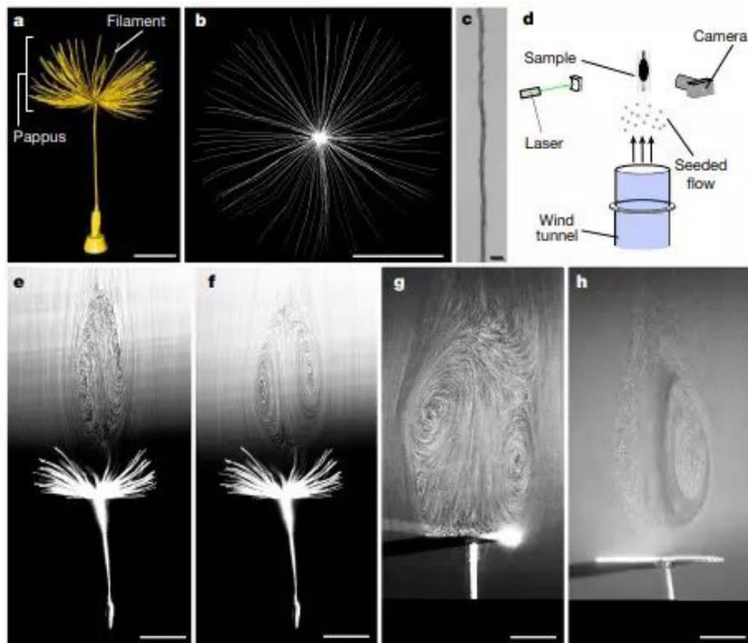
Fig. 2 Airflow analysis of the dandelion flight model
