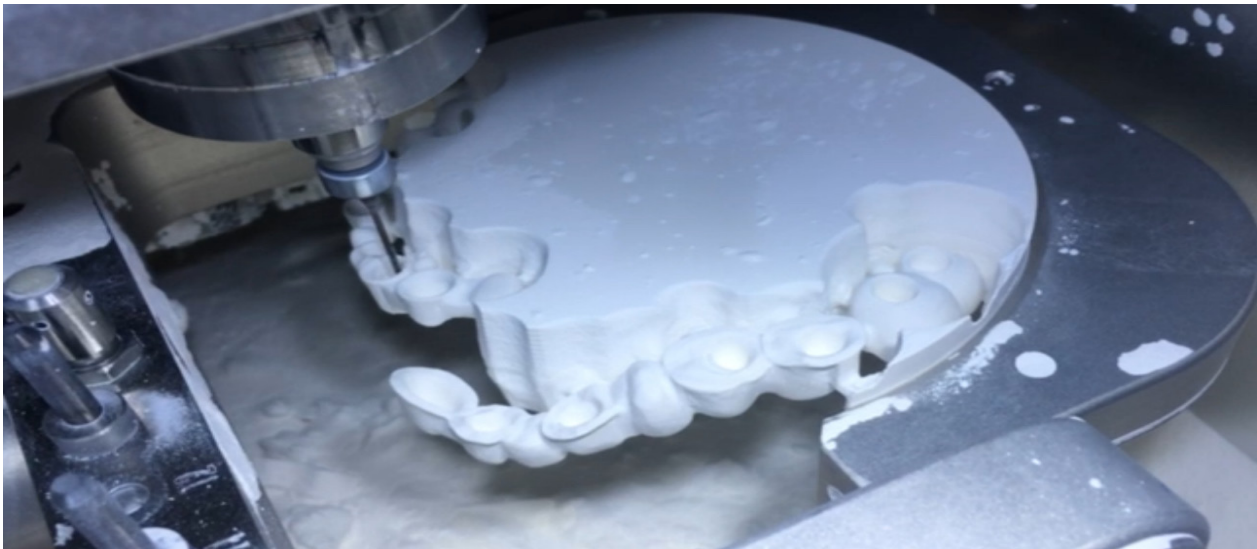
Fig. 1 The zirconia milling process, illustrating the subtractive manufacturing technique used to achieve high precision in durable restorations.
