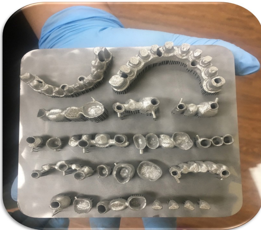
Fig. 3 Completed 3D-printed cobalt-chromium dental restorations, demonstrating the final restoration product. This image highlights the design flexibility of 3D printing, making it particularly advantageous for complex restorative structures.
